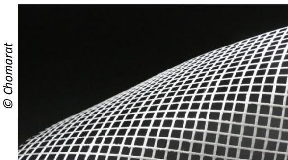
The laid glass scrim was developed in close collaboration with Siniat: *“We designed this glass grid specially to provide good tensile strength and tear resistance. The diameter of the threads is selected to produce a grid with considerable flexibility and mechanical properties. Moreover, the Chomarat coating contributes to the flexibility of the grid and offers excellent resistance to puncture and aging”,* explains Claudio Colombi, product manager for Construction at Chomarat.
