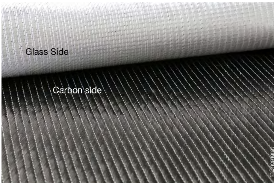
Figure 3 C-PLY™ hybrid structure - carbon/glass
