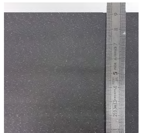
Figure 2 Close-up of 150 ply laminate 92 mm mean thickness Porosity levels lower than 1%
