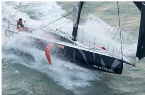
CHOMARAT, the composite reinforcement specialist, has developed a new unidirectional woven tape for its C-TAPE™ line of products. Designed to meet the standards of industrial production, the new C-TAPE™ is reinforcing the foils of the “Figaro Beneteau 3”. These appendages improve the monohull’s stability and performance.
