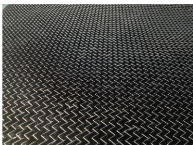
C-PLY™ produced with very heavy tow carbon fiber from ORNL
